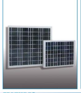
IS10P, IS20P, IS30P, IS40P and IS50P photovoltaic modules are composed of 36 high efficiency polycrystalline cells, manufactured with the most innovative technologies of isotropic texturization and antireflecting coating.
