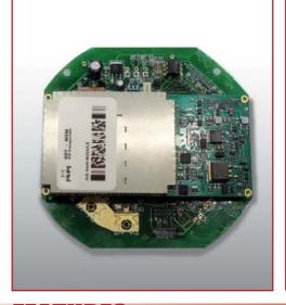
MFAIS circuits are AIS AtoN devices integrated inside our LED lanterns.
