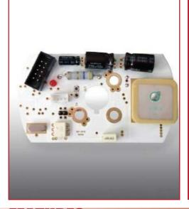
MFGPS position and synchronisation module is a device with double function. On the one hand, it is used to determine buoy positioning and, on the other hand, to synchronise lanterns through a GPS receiver of 12 channels.
