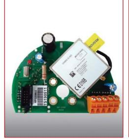
MFGSM circuits are small and compact remote monitoring devices, fitted inside our LED lanterns. The sending and receiving remote control signals is done through GSM mobile phone messages.
