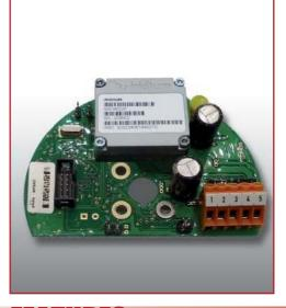
MFSAT circuits are small and compact remote control devices, fitted inside our LED lanterns. The sending and receiving remote control signals is done via satellite.
