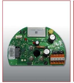
MFUHF circuits are small and compact remote control devices, fitted inside our LED lanterns. The sending and receiving remote control signals is done through UHF frequency radio messages, on freeband.
